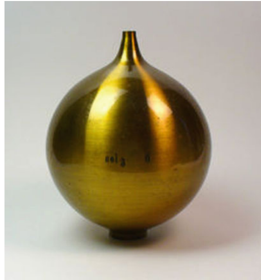
Fig. 3.15 An actual Helmholtz resonator (photo credit: http://en.wikipedia.org/wiki/Hermann_von_Helmholtz )
