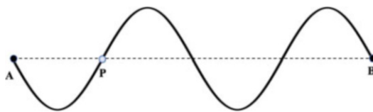
Fig. 12.21 The vibration of the lowest frequency of excitation of the string-harmonic E_7
