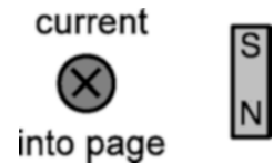
Fig. 5.21 A compass aligns in the opposite direction when the current is flowing into the page
